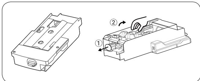
4. After cleaning the tray, put it back in, then firmly push in the icemaker, close the freezer drawer, and switch on the icemaker function via the display panel.
